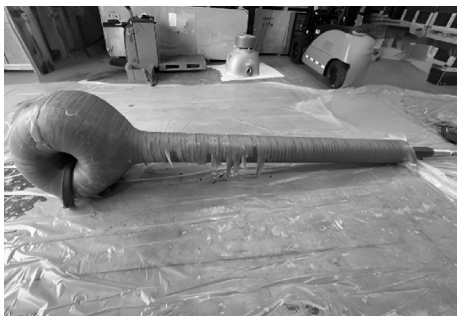
图5 电流互感器器身整体 Fig. 5 Overall body of current transformer
