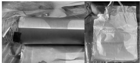
图8 高压屏轻微形变褶皱 Fig. 8 Slight deformation and wrinkling of the high-voltage screen
